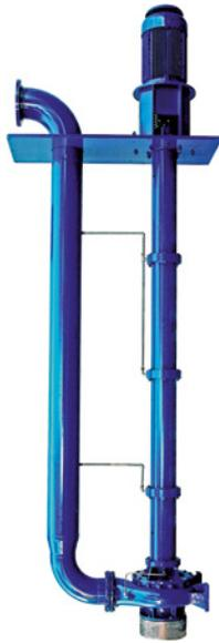
VS pumps are suspended vertical line-shaft, single stage pumps with base plate. The main components are based on MU or MCA serie pumps. They are used to pump clean or dirty fluids that may contain suspended abrasive materials. They are specially useful for many industrial processes, supply drainage, etc.. Thanks to their versatility and material diversification, the VS serie handle and pump a wide range of fluids.
