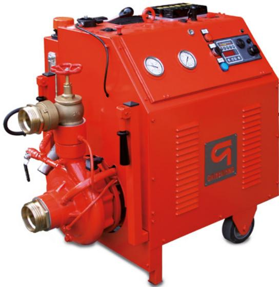
Marine portable diesel engine pump for emergency services, firefighting and drainage. Compact and lightweight construction for easy transportation, it can be pushed by one individual with front wheels, or it can be lifted by two individuals in case of obstacles. Self-priming pump with high suction capacity, designed for pumping seawater. Automatic priming, without need of operator action. Control panel with instruments, manual throttle and engine stop.
