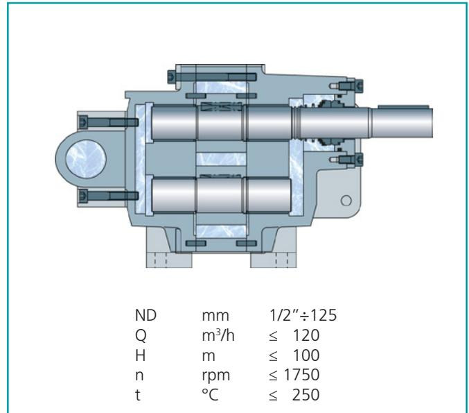
IN pumps are used to pump thick and viscous liquid without suspended solids, at low and high temperature.
