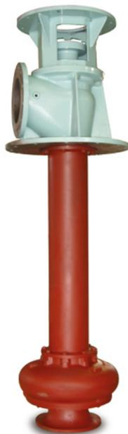
VL are used for main engine lubrication. They are vertical submerged pumps with external motor with base plate for oil pit installation. They have high efficiency closed balanced impeller to reduce load on thrust ball bearing. The concentric diffuser avoids radial load on impeller and makes the pump reliable throughout its operational life. The length of the pump can be sized to the required specific installation. As option VL pumps can have two stages for reaching higher pressures
