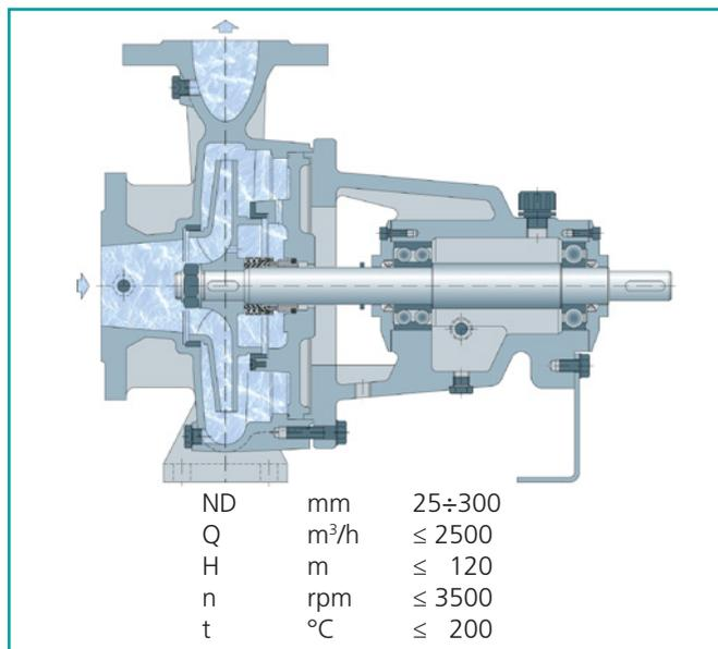
MU pumps are suitable for fresh and sea water, condensate, oils, chemical and petrochemical products in shipbuilding industry, heating plants, air conditioning system, aqueducts, effluent treatment plants, fire fighting, petrochemical plants. Special versions according to Naval Rules (shock-proof, vibration-proof, noise-proof, non magnetic). Further versions: close coupled, selfpriming.
