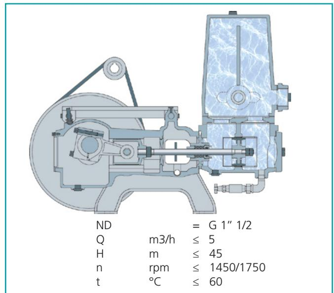
SWL pumps are used for daily bilge, stripping and drainage. They are piston pumps with compact arrangement and high suction capability. The special design of the casing allows a smooth pumping and low pressure pulsations. Low speed and suitably selected materials of construction make the pump particularly reliable for marine duty
