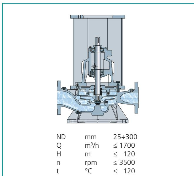
MU-L pumps are suitable for fresh and sea water, condensate, oils, chemical and petrochemical products in shipbuilding industry, heating plants, air conditioning systems, aqueducts, effluent treatment plants, fire fighting, petrochemical plants, scrubber system. Special versions according to Naval Rules (shock-proof, vibration-proof, noise-proof, non magnetic). Further versions: close coupled, selfpriming.
