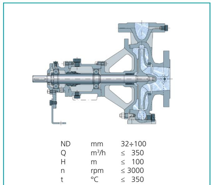
ZN pumps are designed to handle diathermic fluids up to 350°C temperature. Pumped fluids should contain neither abrasive particles nor chemicals which may attack the pump materials. No cooling of the seal chamber required. ZN series pumps are of centrifugal, single stage, horizontal shaft type. Self-balancing impeller by rear impeller blades. The main dimensions of the pump are according to ISO 2858.
