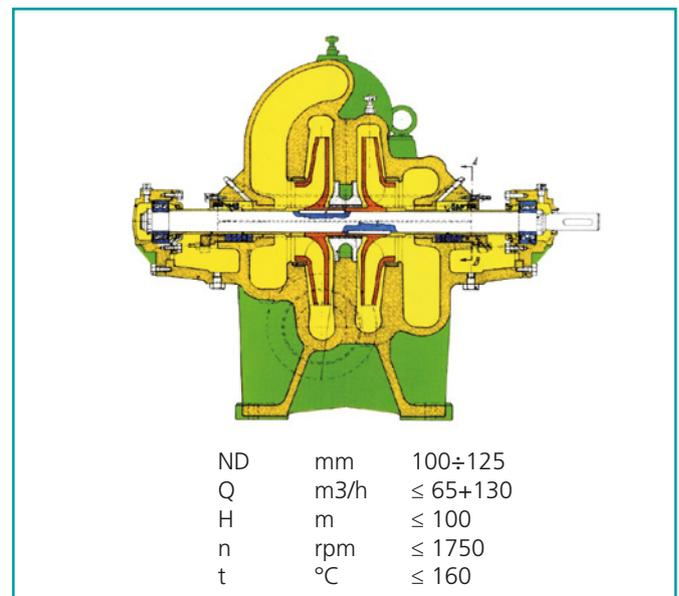
Horizontally split casing centrifugal pumps with two opposite impellers for fire-fighting service. Homologated by the Italian Navy according to UMM 1008 Standards.
